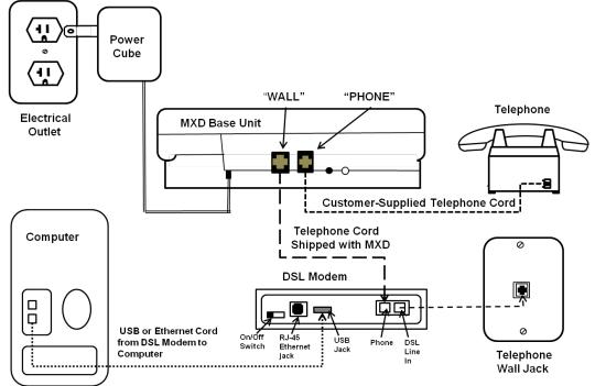
Figure 8. MXD Connection to DSL Modem
