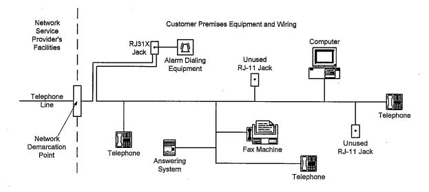
Figure 11. RJ31X Jack Series Installation
