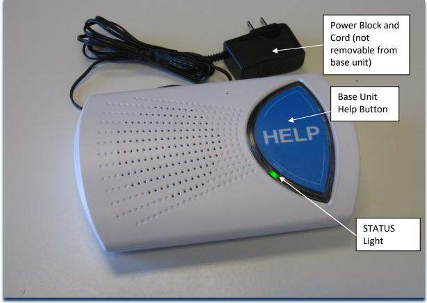
Figure 1. MXD Base Unit and Power Cord
