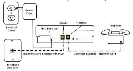
Figure 7. MXD Connections for Locations with Hard-Wired DSL Filters (Connections are the same as for standard telephone service)
