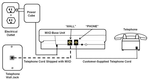
Figure 5. MXD Connections for Traditional (POTS) Telephone Service
